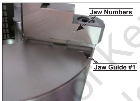
Figure 22. Jaw guides and jaw numbers.
