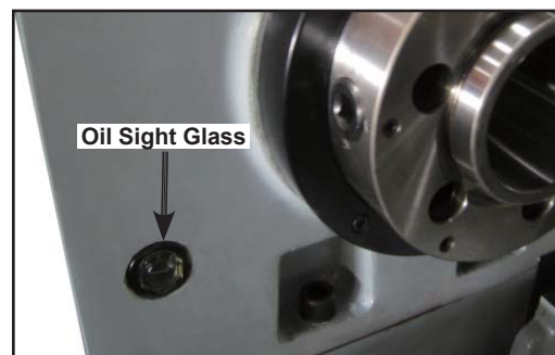
Figure 62. Location of the headstock oil sight glass.
