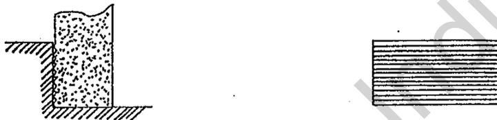
The wheel did not cut to "Relief Angle", thus it contacts the whole face of the work, causing the surface of processing rough and rugged. Also, the greater face of contact will cause burns and cracks.
