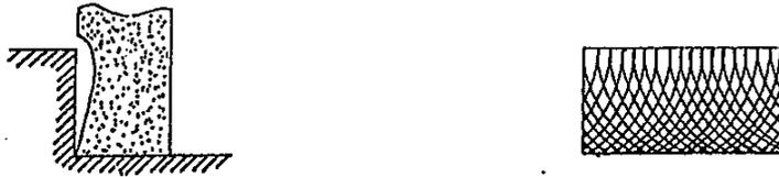
In the case shown in the figure above, the side-grinding wheel and the work have a smaller contact surface, in which case the efficiency is higher, and the surface roughness is better.
