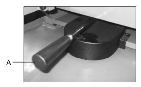
Always lock the horizontal rotation before performing any cutting operation.
