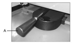
The pivot platform is the structure that holds the saw bow and rotates horizontally for miter cutting up to 60°. Push the lever (A) to right to release and turn bow to the desired angle. After that, push the lever (A) to middle location to lock.
