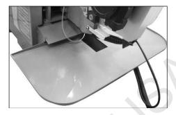
Located above the coolant pump, the spill way is an outlet for the removal of excess chips and debris from the base's tray top. A spray nozzle and hose can be used to washed chips and debris out of the tray, through the tray outlet, and into a receptacle for waste removal.
