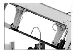
The guide post are the two posts that suspend down from a rail (with width scale), and loosely clamps onto the blade. Their purpose is to keep a blade straight just beyond the dimensions of the material. These guide posts can be repositioned to allow for varying material sizes.
