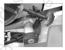
An axle transfer is used to drive the blade brush. The blade brush is designed to clean and help prolonging the life of the blade.
