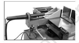
The vise has hydraulic system that allows it to clamp and feed pieces without binding. Fully stroke hydraulic vise can control on control box and clamp material stable. Additionally, the vise seat equipped linear guide to make movement easily.
