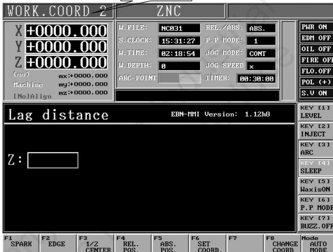
Function Key : Press **[F8]** Coordinate Selection under manual mode for selection Coordinate
