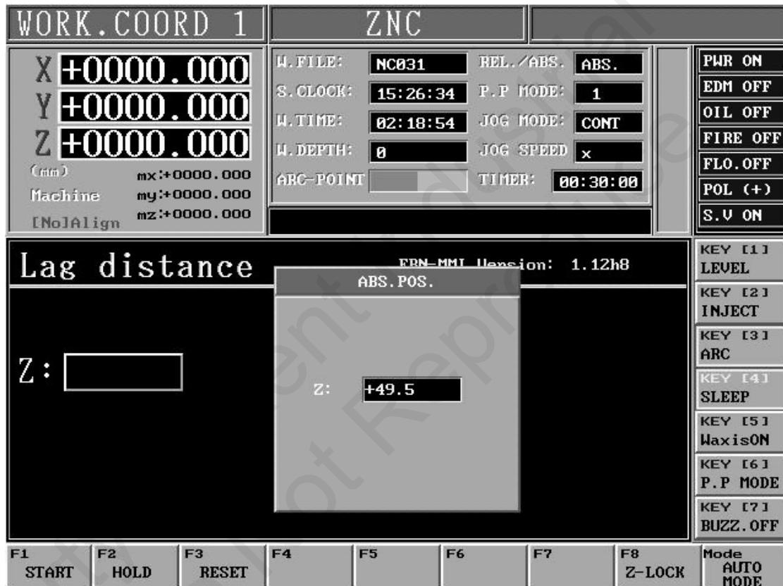
Fig. 6.6 ABS Positioning Screen
