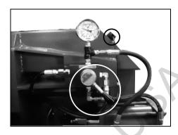
The wheel cover installed a safety micro switch that stop the machine running when the cover was opened.
