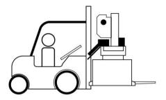
Use a forklift to set machine in position. Sufficient space should be left around the machine to allow safe handling of materials, inspection, and maintenance operations. Take precautions to choose a location that will keep the machine free of vibration and dust caused by other machinery.
