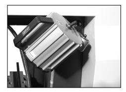
The work light is a light to illuminate work pieces. There is a toggle switch on the top side to turn on/off the work light.
