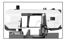
It is sawing mechanism with machine parts consisting of drive members (gears, variable speed, motor, and wheels), tensioning system, light, posts, brush, and guides (blade guards, blade guide blocks).
