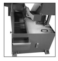
Removable chip tray is for collecting chips and debris.
