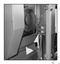
The limit switch -adjusting device stops the saw bow at the bow up or down height. It is activated when the limit switch is contacted by the adjusting stoppers. The stoppers are an adjustable stop that is attached to a vertical bar.
