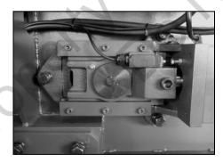
This machine is equipped safety limit switch to prevent continuing damage when a blade has been broken. The safety limit switch will automatically cut power off when there is a loss of tension. Loss of tension may be cause by extreme stretching or breakage of the blade. Loss of power may also occur if the limit switch does not actuate. An adjustment of the tighten bolts are required so that the limit switch's actuator be touched when blade be tensioning.
