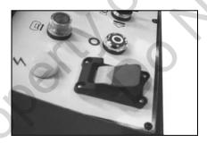
Pull up an attached yellow part to lock the control system. Unless insert it again.
