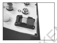
(2) Push up the switch to connect the control power system, and the power light will light on.
