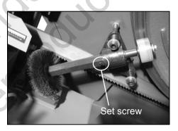
This model has a chip brush driven by a wheel motion directly. The chip brush is designed to clean cutting chips on the blade for prolonging the life of the blade. There is a set screw can be adjusted the brush to touch blade teeth's groove when wire brush worn out.
